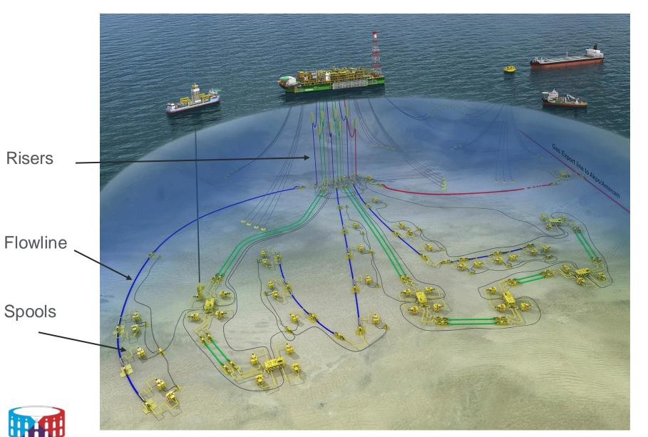
A flowline is a long pipeline (several kilometers long) resting on seabed and linking wellheads to risers.
